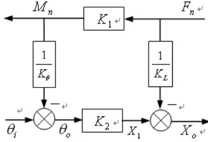
Fig. 4. Deflection block diagram.
