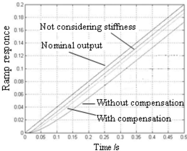
Fig. 7. Ramp response of the feed system.
