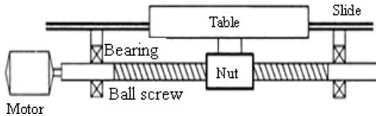
Fig. 1. Schematic diagram of the feed system.
